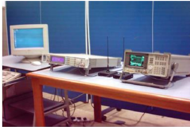
Fig 1: Measurement system: Signal Generator, Spectrum Analyses, Antennas, and Transmission Lines.
