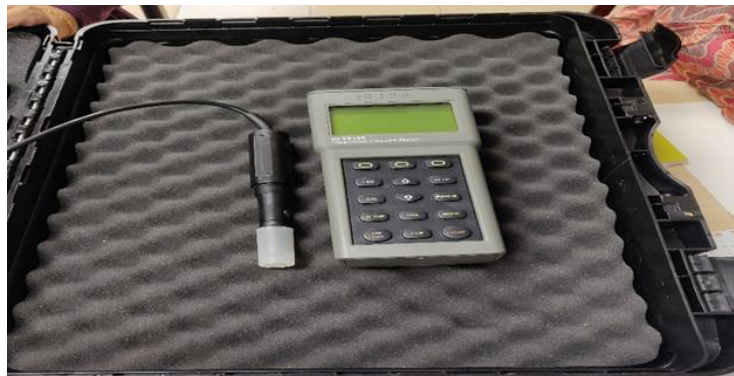
Figure 1.0 Dissolved oxygen meter used to measure the amount of dissolved oxygen in liquid
