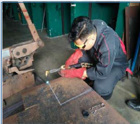
Figure 5(a): The mild steel has been cut by using oxy-acetylene torch.
