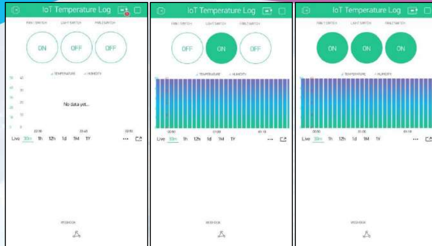
Figure 4.2: Blynk Application displayed Temperature and Humidity Data with Fan and Light Switch Control
