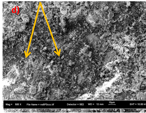
Airborne particle and wear debris superposed on the cracked plateau
