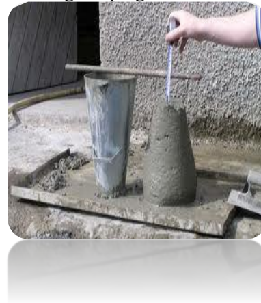
Figure 3 (a): Slump Test Flow Chart Figure 3 (b): Measure the diameter
