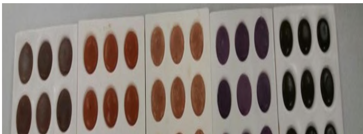
Figure 2: Different plant sources produces different colour. From left: red cabbage, roselle, dragon fruit, beetroot and betel leaf.
