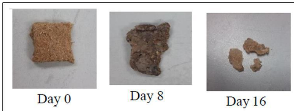
Figure 3: Scanned pictures of the compactness of the foam before and after soil burial test
