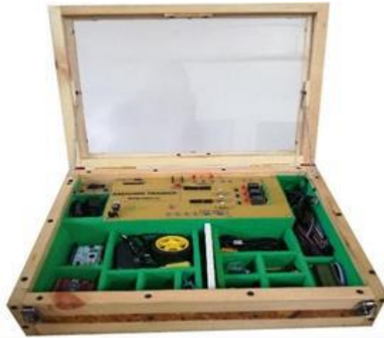
Rajah 5: Model/prototaip Kit Arduino Trainer PTSB Ver 1.0
