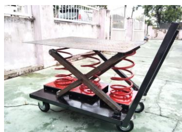
Figure 19: Assembling spring on Trolley Basement and Painting the Trolley
