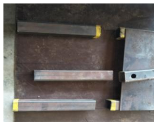
Figure 16: Cutting hollow bar
