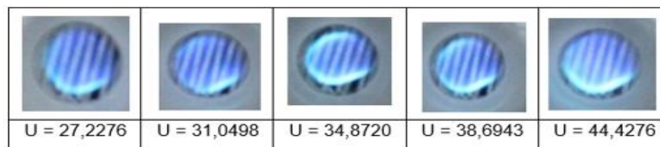
Figure 9: Meso-combustor flame visualization type A with constant U
