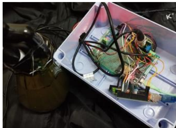
Figure 4: Circuit connection of the Cloud-Based Hydroponic Plant Monitoring System Using Aiven Cloud MySQL Database
