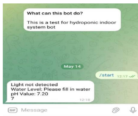
Figure 3: Output from sensor using telegram bot for Indoor Hydroponic System
