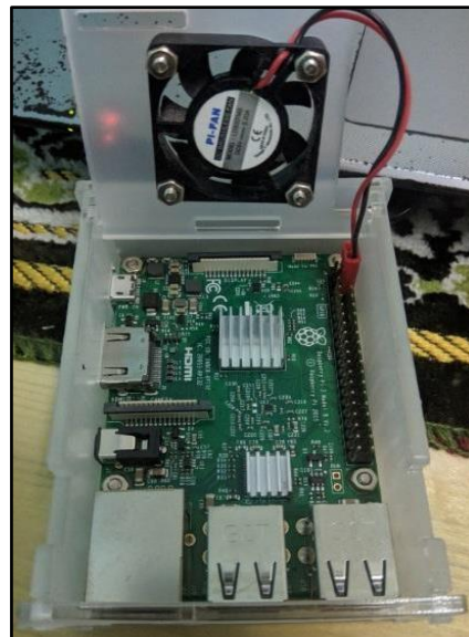
Figure 9: Raspberry Pi 3 Circuit Board
