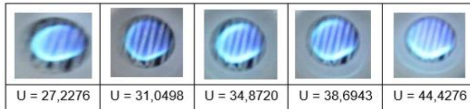
Figure 8: Meso-combustor flame visualization type C with constant U
