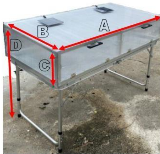
Figure 1: Overall Dimension of Final Product (A:122cm, B:61cm, C: 23cm, D: 77cm)
