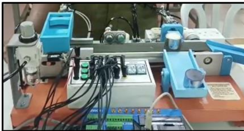
Figure 6: PLC-Based Automatic Mini Conveyor Control System Trainer Final Prototype
