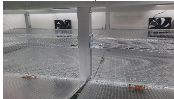
Figure 2: Multiple Removable Stainless-Steel Trays to Hold Fish Samples with Solar Powered Fan
