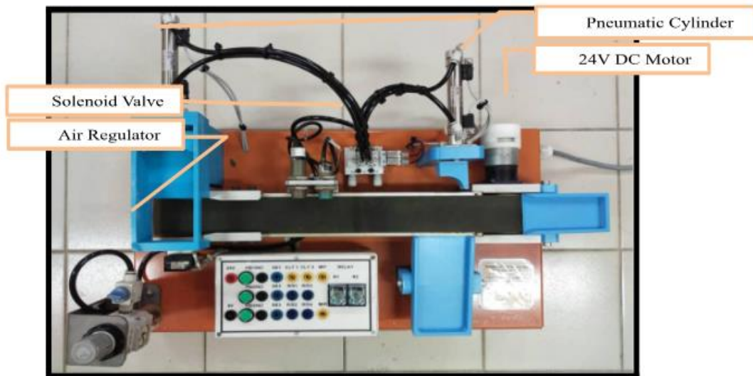
Figure 5: Output components in PLC-Based Automatic Mini Conveyor Control System Trainer Prototype
