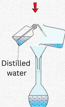
(e) Rinse the funnel with distilled water to ensure all solute enters the flask.
